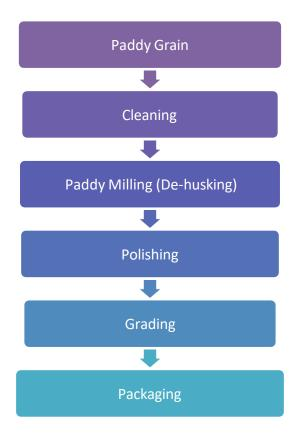
Fig. 1 – Process Flowchart
